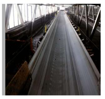
Rubber-fabric oil resistant conveyor belts are manufactured in accordance with WT-6 and are generally made of an EP (polyester-polyamide) fabric ply. At the request of the customer, belts may be made of a PP (polyamidepolyamide) fabric ply.
